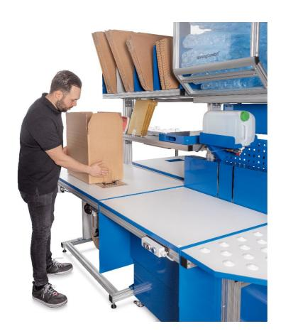
The water-activated tape dispenser for COMFORT.PACK stations is integrated into the surface of the packing table so that shipping cartons can be quickly and easily guided over the dispenser. Image: Storopack
